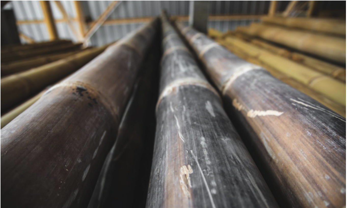
Black Petung for bamboo columns before finishing.
