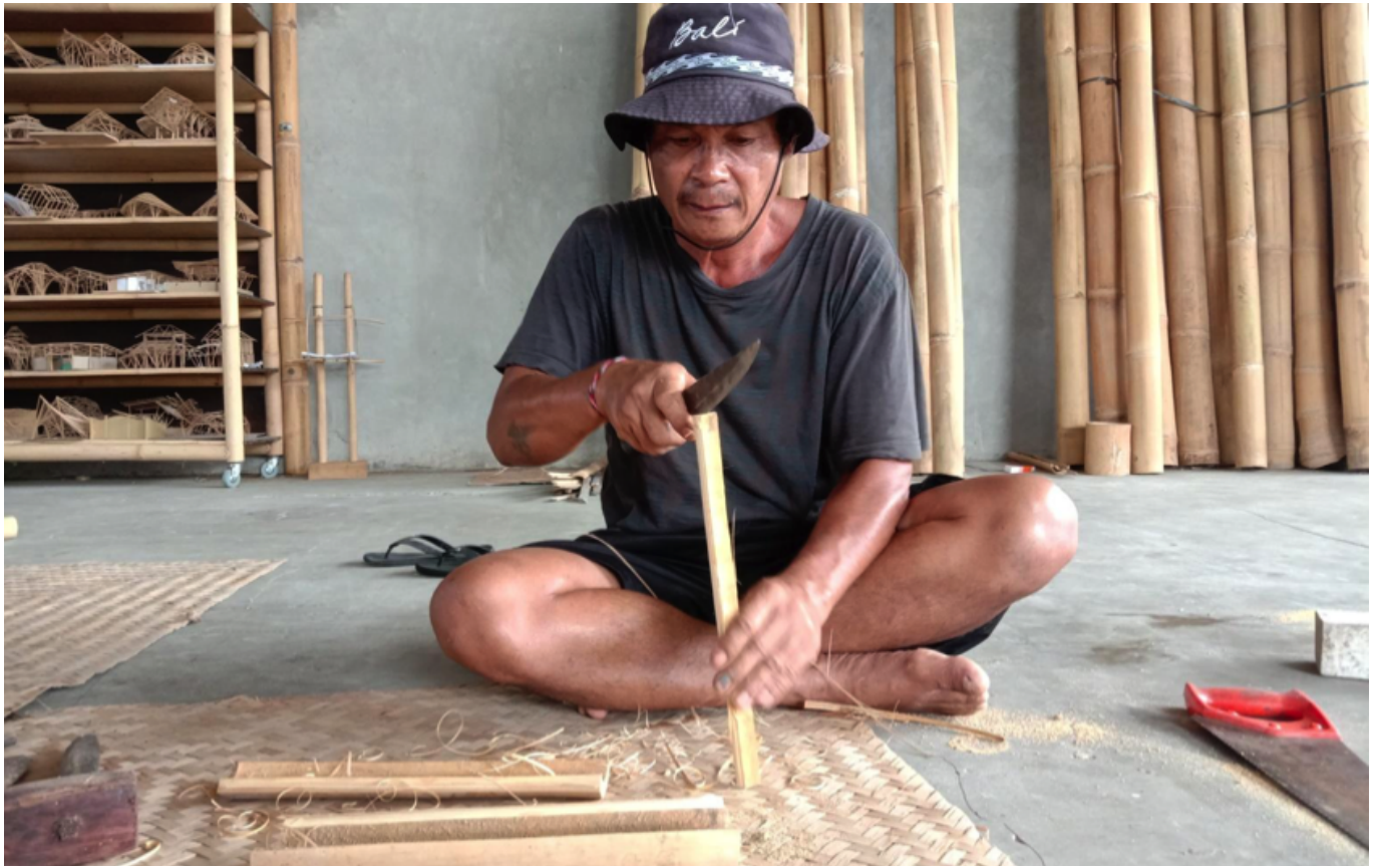
Bamboo pins fabrication process. Asali Bali. 2020.
